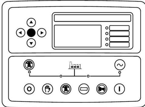
The DSE7310 MKII is an Auto Start Control Module and the DSE7320MKII is an Auto Mains (Utility) Failure Control Module suitable for a wide variety of single, diesel or gas, gen-set applications.
